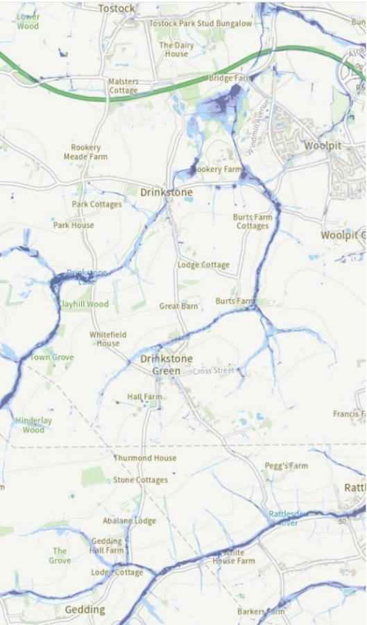
The map identifies where surface water will accumulate for rainfall prediction up to 0.1% AEP (Annual Exceedance Probability) (1in1000). Most of the blue lines will replicate where the existing watercourses/ditches are located. It also identifies areas which are subject to flooding and importantly in the urbanised areas.
